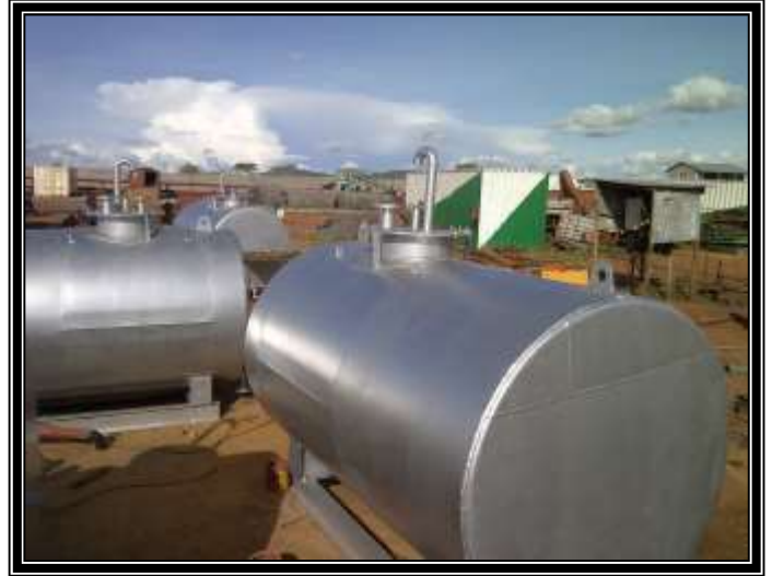
FBRICATION UNHCR DADAAB FUEL TANK
